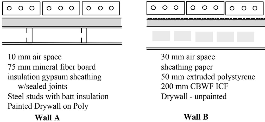
**Figure 4: Horizontal section of test walls (schematic)**
