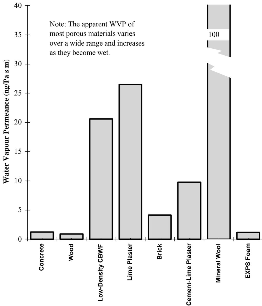
**Figure 1: Water Vapour Permeance of Various Building Materials**
