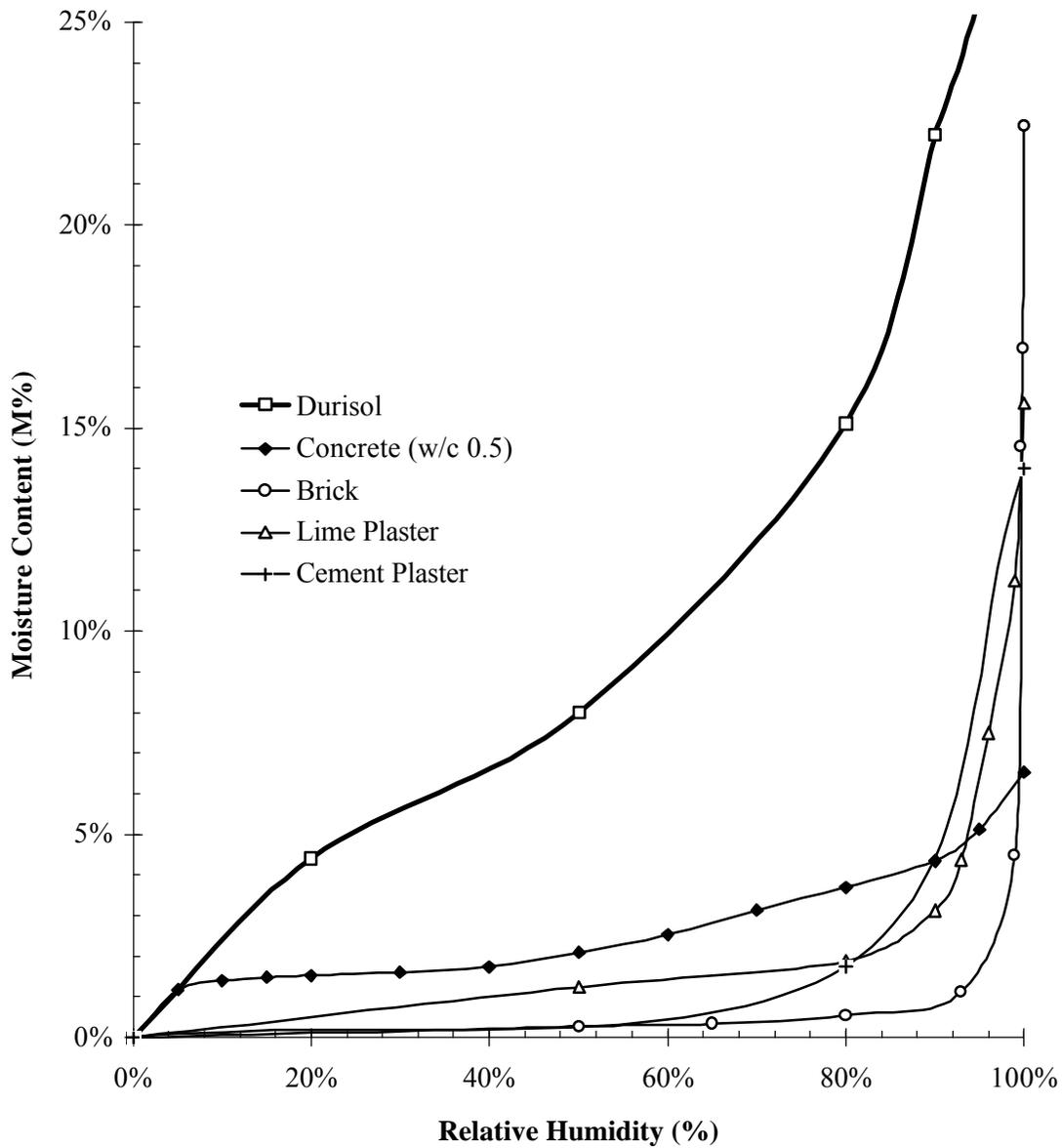
**Figure 2: Sorption Isotherm for Various Building Materials**
